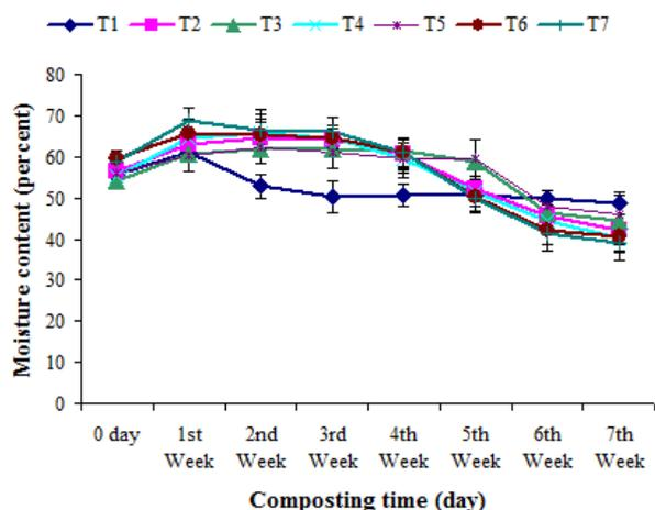
Fig. 1. Changes of Moisture content (%) during composting of press mud. T<sub>1</sub>: Control (Without microorganism); T<sub>2</sub>: PM + *Enterobacter* sp. + CM; T<sub>3</sub>: PM + *Salmonella* sp. + CM; T<sub>4</sub>: PM + *Proteus* sp. + CM; T<sub>5</sub>: PM + *Klebsiella* sp. + CM; T<sub>6</sub>: PM + *Cellulomonas* sp. + CM; T<sub>7</sub>: PM + Consortium + CM
