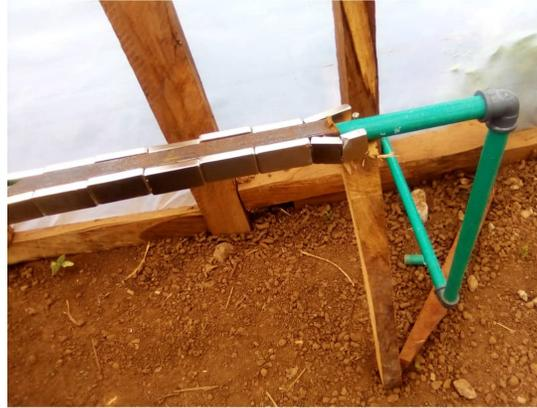
**Figure 3.** Pictorial view of the arrangement of the magnets on the rectangular metallic pipe
